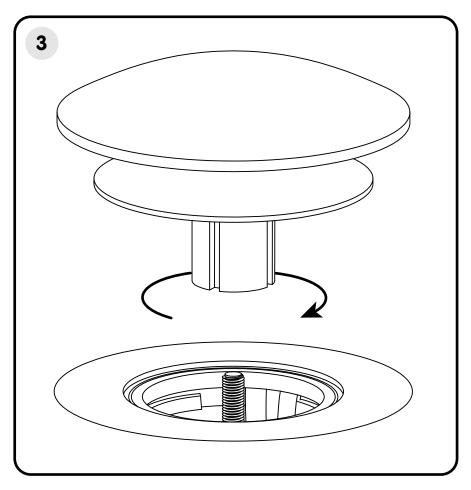
**3.** Fully screw the Converta Plug onto the Round Base. Click the plug a few times to test if the spring is working. Then fill up your basin or bath and test if the plug is working effectively.
