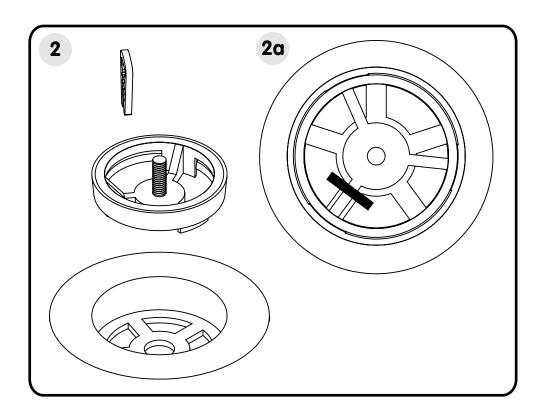
2. Once you have selected the most suitable combination of Round Base and Rubber Ring using the table in Step 1, place the Round Base into the waste and align at least one of the ribs to match up with a rung on the waste.
